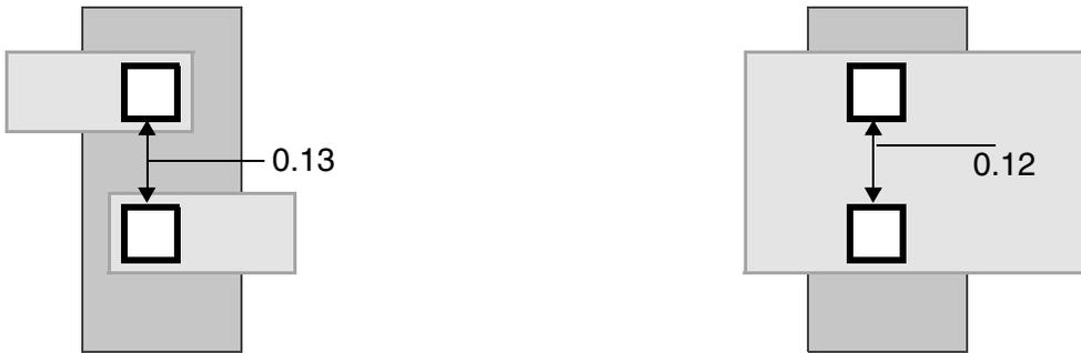
a) Violation, the cuts only share metal shape on one metal layer, and 0.15 parallel overlap spacing is needed. Okay, if EXCEPTSAMEVIA is not used.
